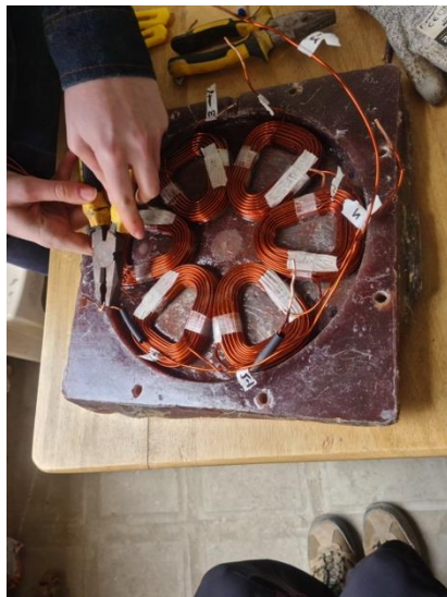
Figure 2- (A) Welding (B) The setup for working with resin (C) Creating the mould for the rotor (D) Filling the rotor mould with coils (E) The blades of carbon fibre and resin
